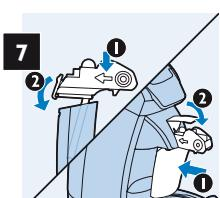
Reattach the lid, place the milk container unit in the machine and press down the lever.
