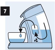
The water in the water reservoir is flushed through the machine and the boiler is filled with water. This process stops automatically, do not interrupt it!
