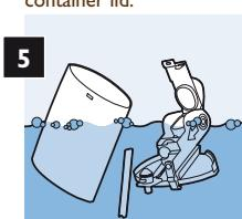
Clean the milk container, milk container lid and milk tube in the dishwasher (recommended) or in hot water with some washing-up liquid. Rinse the parts with fresh water after cleaning.
