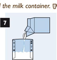
Fill the milk container with cold milk (5-8°C) to the correct level.
