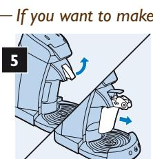
Lift the lever and remove the milk container unit from the machine.
