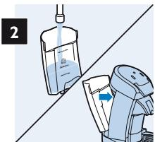
Fill the water reservoir with water and put it back on the machine.
