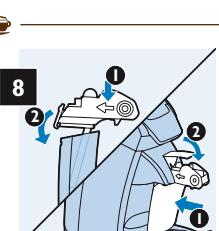
Reattach the lid, place the milk container unit in the machine and press down the lever.
