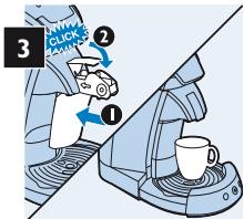
Reinsert the milk container and place an empty cup on the cup tray.
