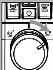
2 Only after adding the descaling solution in the tank, turn the selector switch clockwise to position "C", and then dispense 2-3 cups of water (approx. 150 ml).
