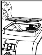
**!** **Only coffee beans must be put into the coffee bean hopper. Ground coffee, instant coffee or any other object may damage the machine.**
