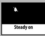
6 When the icon is displayed, rinse the water tank thoroughly and refill it with fresh drinking water.
