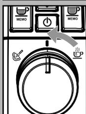
3 Stop dispensing by turning the selector switch back to its central position "0".
