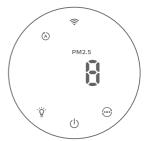
3 Touch and hold the 0 button for 3 seconds to switch off the air purifier.
