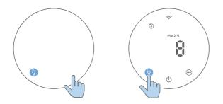
With the light sensor, the control panel can automatically turn on, turn off or dim according to the ambient light. The control panel will be off or dim when the
