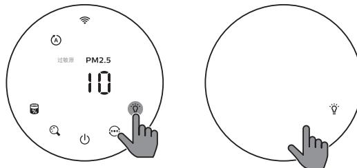
You can touch the light on/off button manually to turn off all lights and the control panel. Touch any button to wake up all lights.
