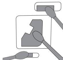
2 Clean the particle sensor with a damp cotton swab. Dry all parts thoroughly with a dry cotton swab.
