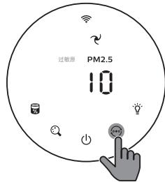
**Gentle mode (Ⓒ):** The air purifier operates at a low speed.
