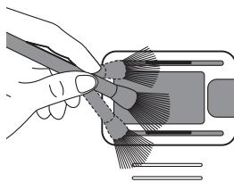
1 Clean the particle sensor inlet and outlet with a soft brush.
