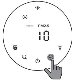
**Auto mode (Ⓐ):** The air purifier automatically adjusts the fan speed in accordance with the ambient air quality.
