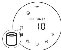
When the filter need to be replaced, the filter replacement alert lights up red.
