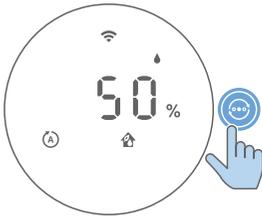
**Auto mode (A):** The appliance automatically adjusts the fan speed in accordance with the ambient air quality.
