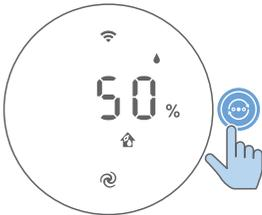
**Turbo mode (🌀):** The appliance operates on the highest speed.
