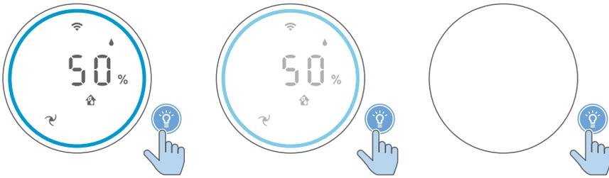
With the light sensor, the control panel can automatically turn on, turn off or dim according to the ambient light. The control panel will be off or dim when the ambient light is dark. You can touch any button to wake up all lights and check the air quality. Then, if no further operation, all lights will be off or dim again to match with the ambient light.
