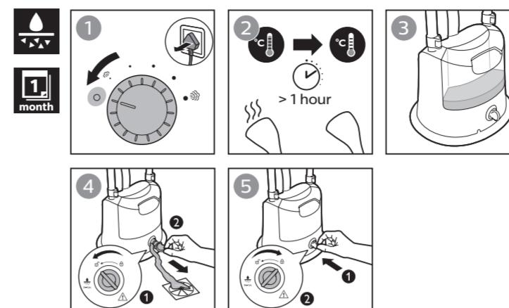
EN To maintain optimal steam performance and prolong the lifetime of the appliance, it is important to remove scales and impurities inside the appliance regularly. Therefore, it is recommended to perform the de-calc process at least once a month.
