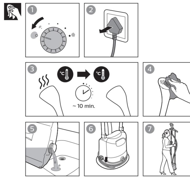
EN **Note:** Clean the appliance and wipe any deposits off the steamer head with a damp cloth and non-abrasive liquid cleaning agent. Always empty the water tank after usage, to prevent calc build-up and maintain good steam performance.
