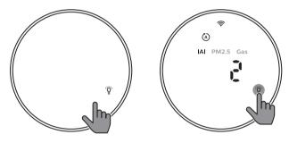
With the light sensor, the control panel can automatically turn on, turn off or dim according to the ambient light. The control panel will be off or dim when the ambient light is dark. You can touch any button to wake up all lights. Then, if no further operation, all lights will be off or dim again to match with the ambient light.
