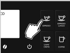
**9** Coffee brewing automatically stops when the preset level is reached; however, you can stop it earlier by pressing the same button of the selected beverage.
