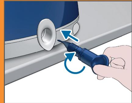
When no more water comes out, reinsert the EASY DE-CALC knob and turn it clockwise to tighten it.
