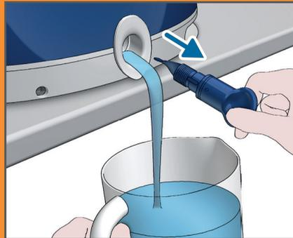
Remove the EASY DE-CALC knob and let the water with scale particles flow into the cup.
