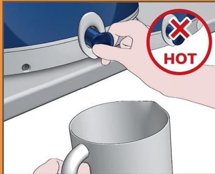
Place the steam generator at the edge of a table or sink and hold a cup under the EASY DE-CALC knob.
