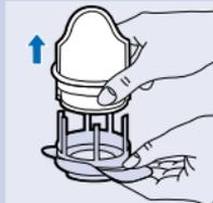
**1** Slide the ring holding the edge of the dustbag upwards and remove the old dustbag.
