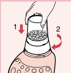
**4** Turn the assembled mill upside down and screw it onto the motor unit in the direction of the arrow.
