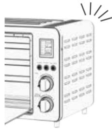
2. Before plugging in the power, please check if the power is 220-240V/50/60Hz. After plugging, the screen is lit for 2 seconds and device is ready to use post 3 buzzer sounds. The default selection is "bake", the default temperature is displayed as 180°C, and the default time is displayed as 30 mins.
