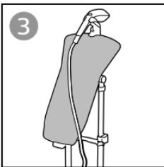
**EN** To adjust the height of the pole, ensure that board tilting lever is in locked position before attaching the board lock to the poles.
