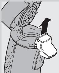
**4** Take the coffee spout out of the machine by sliding it upwards.
