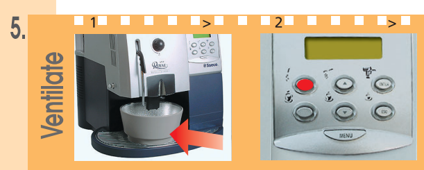
5. Ventilate 1 Place receptacle under nozzle 2 Draw off hot water until no more air escapes
