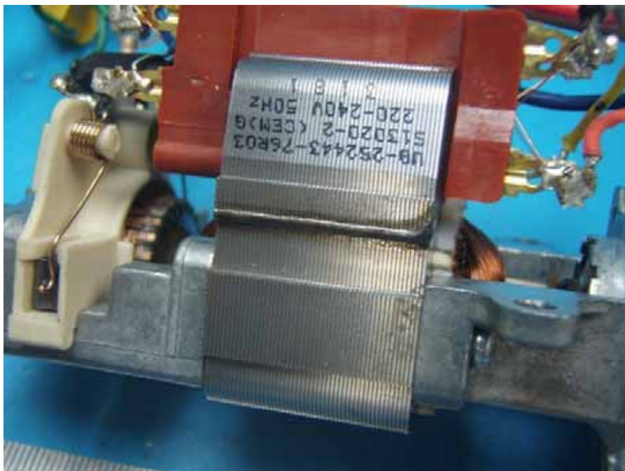
AC motor of HV version (ECM motor)
