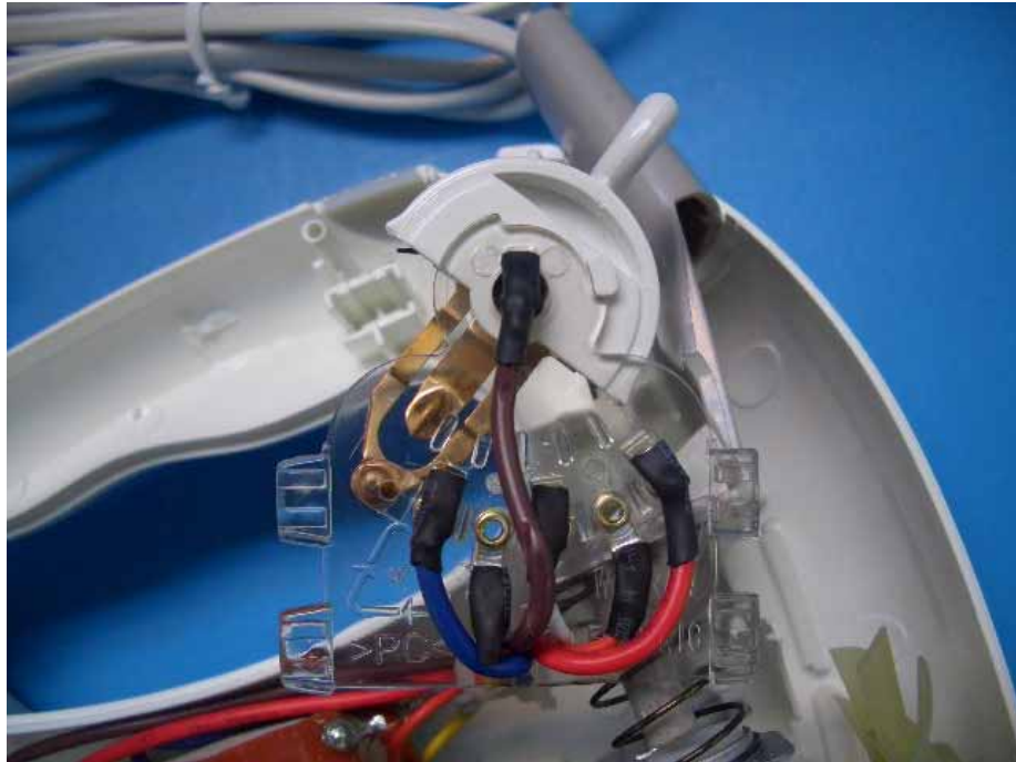
Switch construction ((HR1458 with remove the turbo switch)
