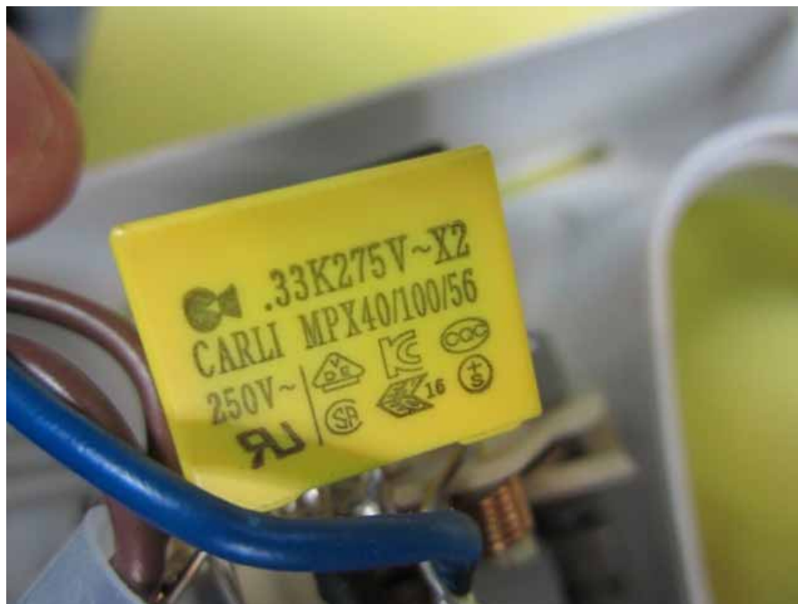
Alternative X-capacitor (0,33 \mu F) for HV version models with ECM UB-252443-76R03 motor only
