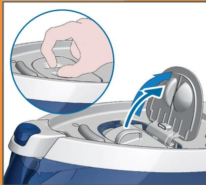
Remove the iron from the iron platform and open the ANTI-CALC cartridge compartment.
