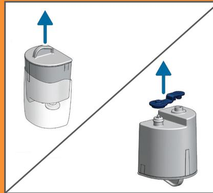
Pull out the rubber cap from the bottom of the ANTI-CALC cartridge.
