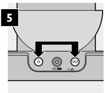
Put a bowl with a capacity of least 1500 ml under the spout to collect the descaling mixture. Press ▷ and ▷ simultaneously to start descaling. Hot water comes out at intervals! The machine stops descaling 3 to 4 times to let the descaler mixture act and to heat up. Let the machine complete the entire descaling cycle, which takes 4 to 5 minutes. Do not switch off the machine during the descaling cycle!
