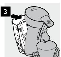
Put the water reservoir back onto the coffee machine.
