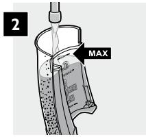
Fill the water reservoir with water up to the MAX indication.
