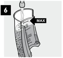
Flush the machine with fresh water. Fill the water reservoir with fresh tap water up to the MAX indication and repeat steps 3 to 5. Do this two times.
