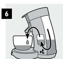
The machine fills itself with water and hums loudly in the process. This process stops automatically, do not interrupt it!
