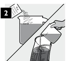
Mix 50 grams of citric acid with 1 litre of water. Fill the water reservoir with the descaler mixture.
