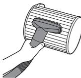
3 Clean the surface of the filter with a vacuum cleaner.
