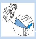
For optimal performance of the machine, lubricate the brewing unit after it has brewed 500 cups of coffee or once every 3 months. Contact the Philips Saeco hotline to buy lubricant.
