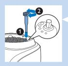
You can adjust the grinding degree of the machine. At each grinding degree selected, the ceramic coffee grinder guarantees a perfectly even grind for every cup of coffee you brew. It preserves the full coffee aroma and delivers the perfect taste to every cup.
