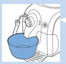
During the manual rinsing cycle, the machine brews one cup of coffee to prepare the inner circuit for use.
