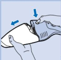
Replace the filter if it can no longer be cleaned properly (usually after having been cleaned 50 times).
