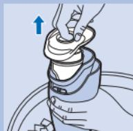
Empty the dust compartment and clean the filter regularly.
