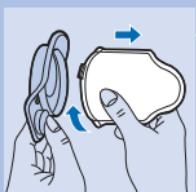
**3** Gently turn the filter clockwise to detach it from the frame.
