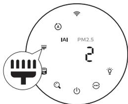
Clean the surface of filter with vacuum cleaner when the filter cleaning alert
