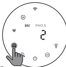
7 Touch and hold the filter status check/reset button
