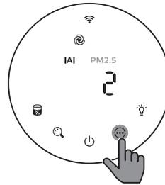
**Turbo mode (
