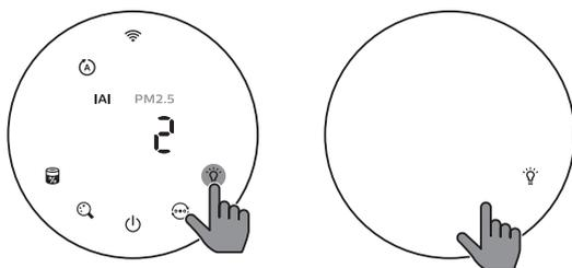
You can touch the light on/off button
