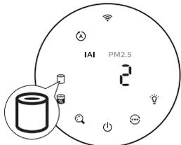
When the filter need to be replaced, the filter replacement alert
