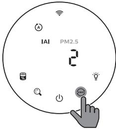
**Auto mode (
