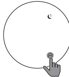
**Sleep mode (
