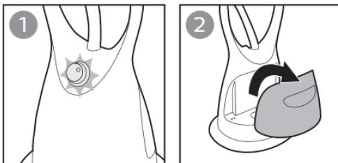
**EN** Refill the water tank and insert it back. You can resume steaming after turning the steam knob. The ring should stop flashing.
