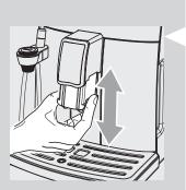
The height of the dispensing spout can be adjusted to better fit the dimensions of the espresso cups that you wish to use.
