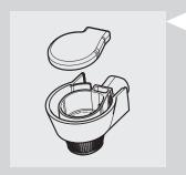
21 Remove the rubber cover as shown in the picture.
