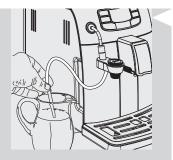
4 Insert the suction tube in the milk container.
