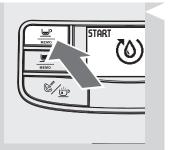
2 Press the " button to start the cycle. The machine starts the automatic priming of the circuit by dispensing some water through the steam wand.
