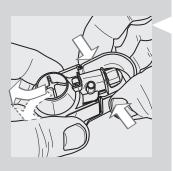
**20** To detach the Automatic Milk Frother, press the sides and remove it by applying light lateral movements as shown in the figure.
