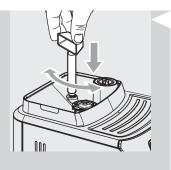
1 Press and turn the grinder adjustment knob one notch at a time. You will taste the difference after brewing 2-3 cups of coffee.
