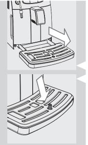
3 Empty and clean the drip tray. Perform this operation also when the full drip tray indicator is raised.
