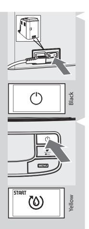
12 Switch the power button to "I" to turn on the machine. The display shows the stand-by icon.
