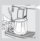
When warm-up is completed, the machine automatically performs a rinse/self- cleaning cycle of the internal circuit with fresh water. This takes less than a minute.
