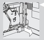
2 Empty and clean the coffee residues drawer located inside of the machine. Open the service door, remove the coffee residues drawer and empty the coffee grounds.
