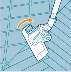
2 To clean hard floors, push the rocker switch on top of the nozzle backwards with your foot. The brush strip for cleaning hard floors comes out of the nozzle housing.
