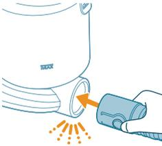
**1** To connect the hose, insert it into the hose connection opening until it snaps into place.
