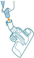
4 To disconnect the nozzle from the tube, push the nozzle with one hand and pull the tube out of the nozzle with the other hand.
