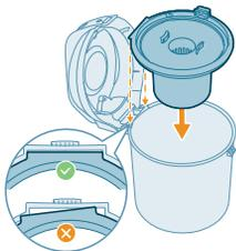
11 Properly install the Vortex finder by ensuring it fits securely against the edge of the dust bucket, as shown in the illustration.
