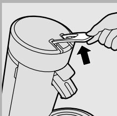
**3** Release the lid by moving the lever upwards.
