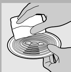
**7** Rinse the parts with fresh water after cleaning and put them back into the machine.
