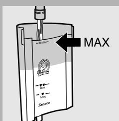
Regular descaling will prolong the life of the coffee machine and will guarantee optimal brewing results for a long time. If the machine is used twice a day on average, it must be descaled once every 3 months.
