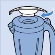
To avoid spillage, always assemble the stopper with securing clip onto the lid before you start processing.
