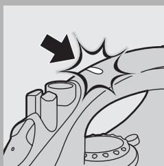
An electronic safety device will automatically switch the heating element off if the iron has not been moved for a while.
