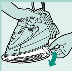
**1** Type GC4340 only: remove the heat-resistant protective cover. Do not leave the heat-resistant protective cover on the soleplate during ironing.
