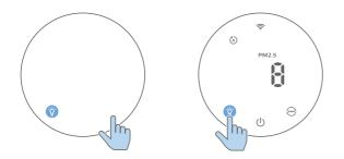
With the light sensor, the control panel can automatically turn on, turn off or dim according to the ambient light. The control panel will be off or dim when the ambient light is dark. You can touch any button to wake up all lights. Then, if no
