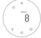
3 Touch and hold the 🕐 button for 3 seconds to switch off the air purifier.
