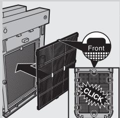
**8** Put filter 1 (pre-filter) back into the appliance.
