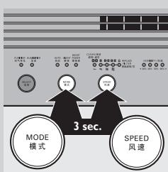
adjust the sensitivity of the air quality sensor. The default setting of the air quality sensor is standard sensitivity.
