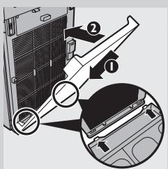
**9** To reattach the front panel, insert the two hooks at the bottom of the front panel into the openings at the bottom of the appliance first (1). Then push the panel against the body of the appliance (2).
