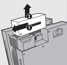
**1** Slide the water bucket cover at the back of the appliance to the left (1) and remove it from the appliance (2).
