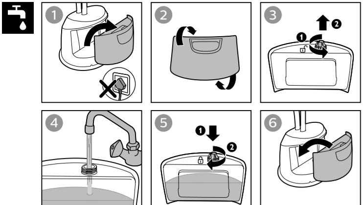
**EN** Your appliance has been designed to be used with tap water. In case you live in an area with hard water, fast scale build-up may occur. Therefore, it is recommended to use water without minerals such as distilled or purified water to prolong the lifetime of your appliance.
