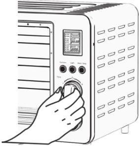
4. If you need to adjust "Time" and "Temp", after "Preset Menu" is selected using function button, turn the "Time" knob to set the time, and turn the "Temp" knob to set the temperature. After this press the "Start/Stop" button to confirm and start cooking
