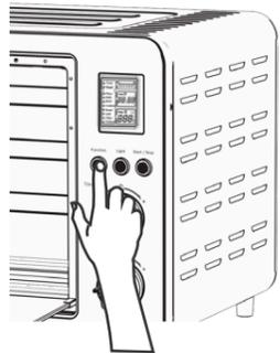
3. Press the "Function" button to select the required menu, and default "Time" and "Temperature" are displayed according to the selected menu. Press the "Start/Stop" button to start working
