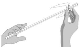
2. Rotate the skewer screw to fix the spit rod at the proper position
