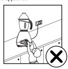
Always ensure that speed selector knob is at '0' position before fixing accessories.
