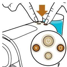
8 The ristretto button starts to flash quickly. Press the ristretto button to activate the descaling cycle. The machine dispenses the entire descaling solution at regular intervals. This takes up to 30 minutes.
