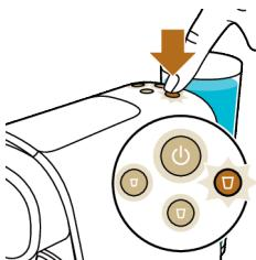
**11** Press the lungo button to start the flushing cycle.
