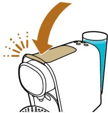
6 Place a bowl with a minimum capacity of 1.5 liters on the lower drip tray under the coffee dispensing spout to collect the descaling solution.
