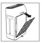
3 Wash the pre-filter under a running tap. If the pre-filter is very dirty, use a soft brush to brush away the dust.
