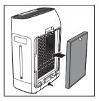
5 Put the pre-filter back into the appliance, mount the pre-filter onto the bottom of the appliance first, and then push the clip on the top of pre-filter against the appliance.
