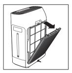
To remove the pre-filter, press the clip down and pull the filter towards you.
