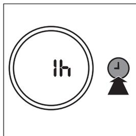
↳ For **AC3252**, the timer is available in **1, 4 or 8** hours. For **AC3254** and **AC3256**, the timer is available from **1 to 24** hours.
