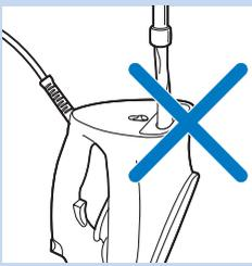
Do not pour water, vinegar, descaling agents or other chemicals into the iron from the opening of the Quick Calc Release.
