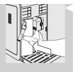
5 Push gently on the edge of the water tank door to release the hand-
