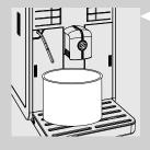
**9** Press the " $\stackrel{\square}{=}$ " button to start the descaling cycle.
