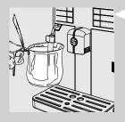
2 Press the "" button to start the cycle. The machine starts the automatic priming of the circuit by dispensing some water through the Classic Milk Frother.
