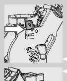
10 Make sure the hook to lock the brew group is in the correct position by firmly pressing the "PUSH" button until it locks into place. Check if the hook is at the top end position. If it is not, please try again.
