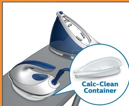
Place the iron on the Calc-Clean container on an even, stable surface.
