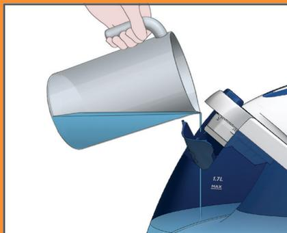
Fill the water tank halfway and switch on the appliance.
