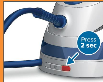
Press and hold the '**CALC CLEAN**' button for **2 seconds** until you hear short beeps.
