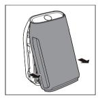
Press the two clips down (1) and pull the pre-filter towards you (2).
