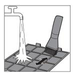
Allow the pre-filter to air dry thoroughly before placing back in the air purifier.
