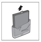
5 Place the filter (FY1417) into the air purifier.
