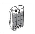
4 If the pre-filter is very dirty, use a soft brush to brush away the dust . Then wash the pre-filter under running tap water.
