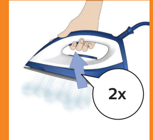
For a steam boost, double press the trigger in quick succession.
