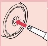
**1** Push the driving shaft of the mixing bowl into the opening of the mixing bowl from below. You will hear a click when it snaps into place.
