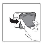
3 Clean the sensor, the dust inlet and outlet with a lightly moistened cotton swab, and finish with a dry cotton swab.
