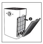
7 Repeat the above steps and assemble the air purification filters for the other side of the appliance.
