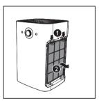
4 Put the unpacked air purification filters into the appliance.
