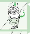
3 Screw the blade unit onto the beaker.
