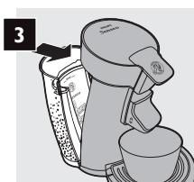
3 Put the water reservoir back onto the coffee machine.
