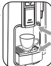
Cup for filter coffee ☕ or cappuccino ☕: coffee dispensing spout raised and drip tray in the outer position.
