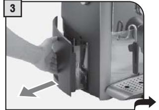
Remove the water tank. We recommend installing the "Aqua Prima" water filter (see page 11).
