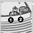
2 The reference marks inside the coffee bean hopper indicate the grind setting. There are 5 different grind settings to choose from position 1 for coarse grind - lighter taste to position 2 for fine grind - bolder taste
