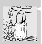
When warm-up is complete, the machine automatically performs a rinse/self-cleaning cycle of the internal circuit with fresh water. This takes less than a minute.
