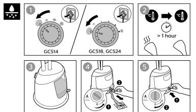
**EN** To maintain optimal steam performance and prolong the lifetime of the appliance, it is important to remove scales and impurities inside the appliance regularly. Therefore, it is recommended to perform the de-calc process at least once a month.
