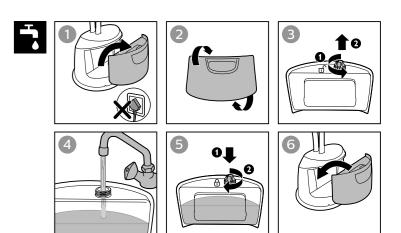
Your appliance has been designed to be used with tap water. In case you live in an area with hard water fast scale build-up may occur. Therefore, it is recommended to use water without minerals such as distilled or purified water to prolong the lifetime of your appliance.
